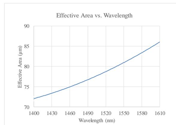
**Figure 1: Effective area vs the wavelength of the typical telecom single mode fiber.**
