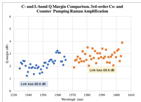
**Figure 12: Measured Q values for the optimal co- and counter pumping conditions.**
