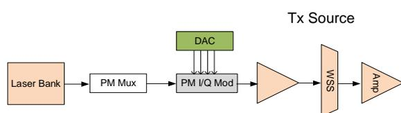
**Figure 7: Transmitter source details**
