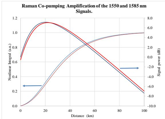
**Figure 4: Comparison of co-pumping Raman amplification of single C-band (1550 nm) and L-band (1585 nm) signals by a single 600-mW pump at 1450 or 1485 nm, respectively.**
