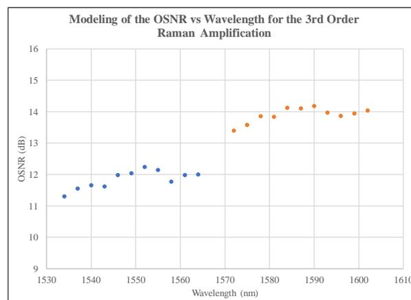
**Figure 3: 3rd-order Raman counter pumping modeling – comparing C- and L-band OSNR in the 300 km PSCF link.**
