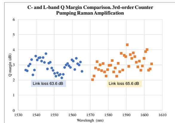
**Figure 11: Measured Q margin values for the optimal counter Raman pumping conditions.**
