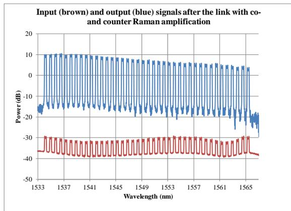
**Figure 9: Spectrum of signals at input and output of the C-band link**
