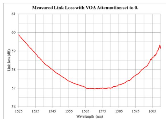
**Figure 6: Measured losses in the 310 km of the PSCF used in the experiments when middle-stage VOA was set to 0.**
