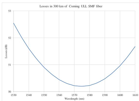
**Figure 2: Losses of a 300 km link of Corning ULL SMF fiber**
