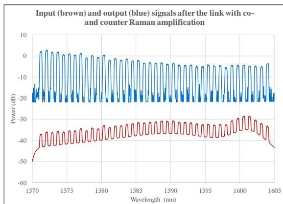
**Figure 10: Spectrum of signals at input and output of the L-band link**
