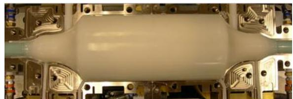
**Figure 6: Polyethylene insulation molded over splicebox**
