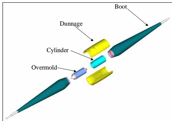
**Figure 2: Example universal Armorless Joint**
