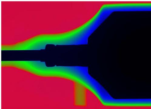
**Image 4: Coloured contouring of wall thickness of an X-ray moulded joint**
