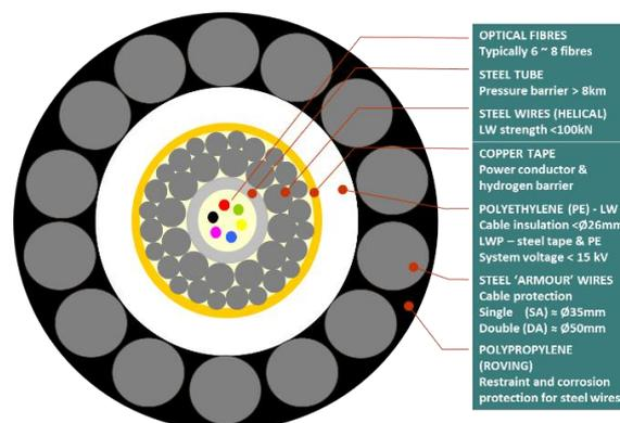
**Figure 1: Typical repeated Cable**
