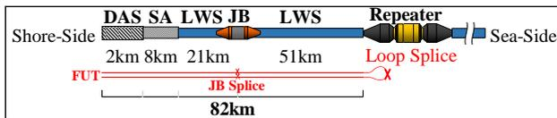
**Figure 7: Submarine Cable Configuration, as Laid**
