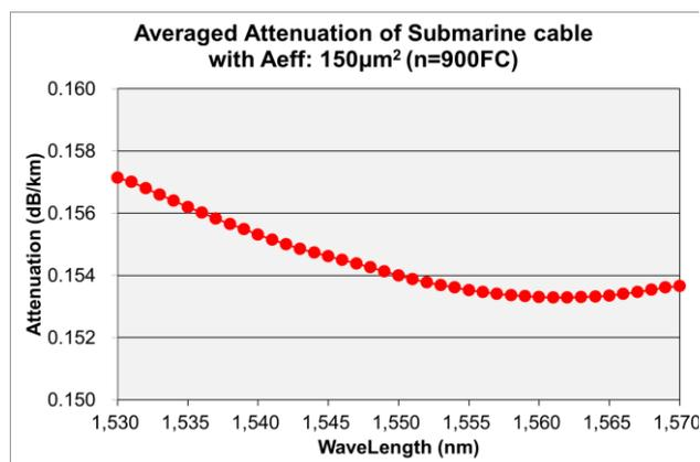
**Figure 4: Averaged Attenuation vs Wavelength (Aeff: 150µm<sup>2</sup>)**
