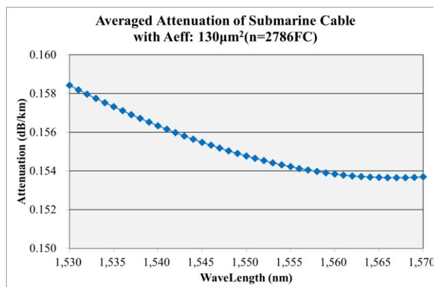
**Figure 3: Averaged Attenuation vs Wavelength (Aeff: 130µm<sup>2</sup>)**
