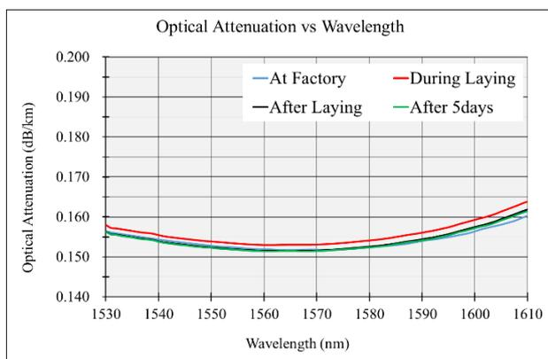
**Figure 10: Optical Attenuation vs Wavelength**
