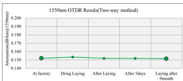
**Figure 11: 1550nm OTDR Results (Two-way method)**
