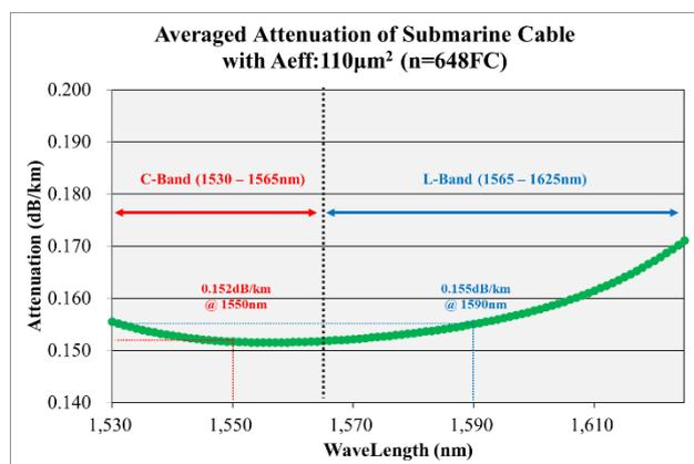
**Figure 5: Averaged C+L band Attenuation vs Wavelength (Aeff: 110µm<sup>2</sup>)**
