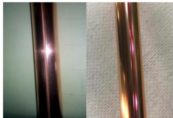
**Figure 9: Comparison of welding process (laser weld to left, argon arc weld to right)**
