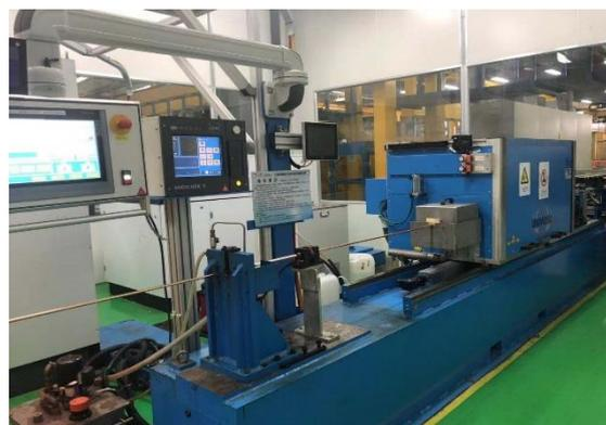
**Figure 2: Laser welding line**
