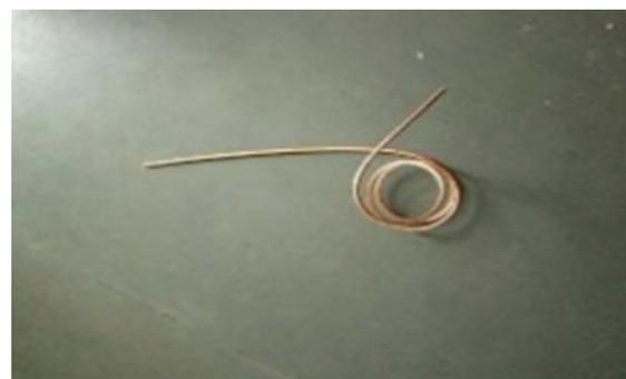
**Figure 7: Bending wrap test**
