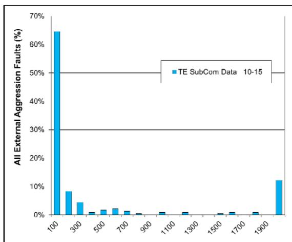
**Figure 2: Depth distribution in meters of all external aggressions faults** [2]
