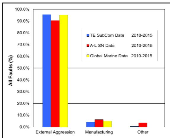
**Figure 1: Overall causes of fiber optic cable failures** [1]
