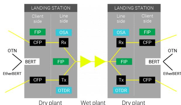
**Figure 3: Location of typical testing**
