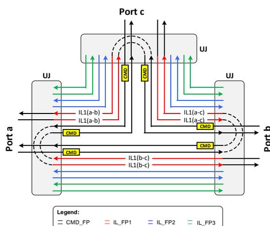
**Figure 12: Symmetrical Design of Spare BU (for BU1 replacement)**
