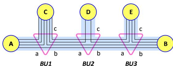
**Figure 1: Fiber Routing of BU in Multi-branch System**
