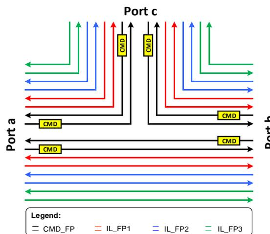
**Figure 6: Optical Architecture of Spare BU**
