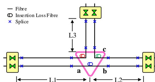
**Figure 2: Optical Powering Design and Insertion Loss Compensation Diagram**
