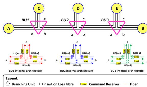
**Figure 5: Optical Architecture for 2 Fiber Pair Repeatered System with 3 BUs**
