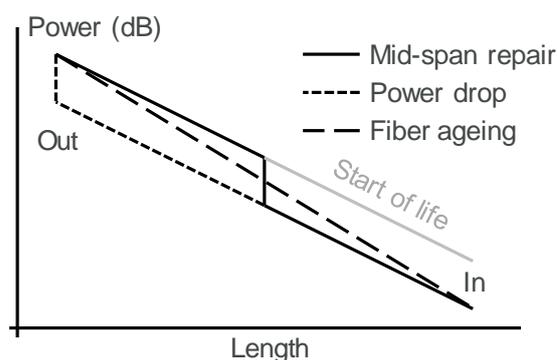
**Figure 1: Power profile along a fiber section**
