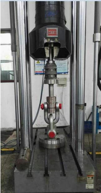
**Figure 4: Engineering tension facility setup for investment castings**
