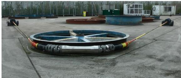
**Figure 5: Round the sheave testing on castings @ 200KN**
