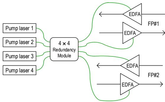
**Figure 3: 4x4 Pump-redundancy Scheme**
