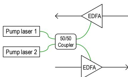
**Figure 1:  $2 \times 2$  Pump-redundancy Scheme**
