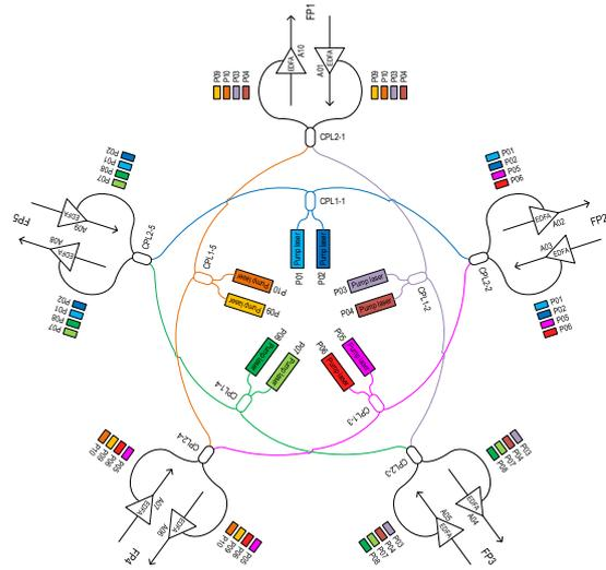
**Figure 6: Two EDFAs in Each Fiber Pair Powered by the Same Pump Lasers**
