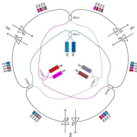
**Figure 7: 3FP Repeater Pump-redundancy Scheme**
