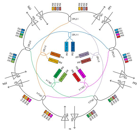
**Figure 5: Planar Graph of 5FP Repeater Pump-redundancy Scheme**
