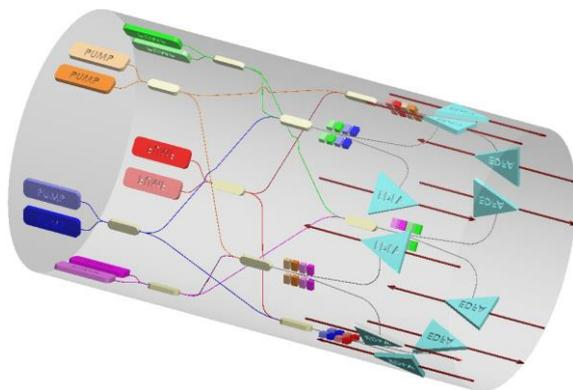
**Figure 4: Novel Pump-redundancy Scheme of Five Fiber-Pair (5FP) Repeater**
