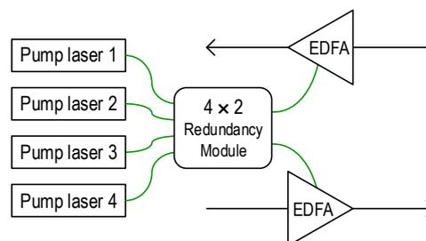
**Figure 2:  $4 \times 2$  Pump-redundancy Scheme**
