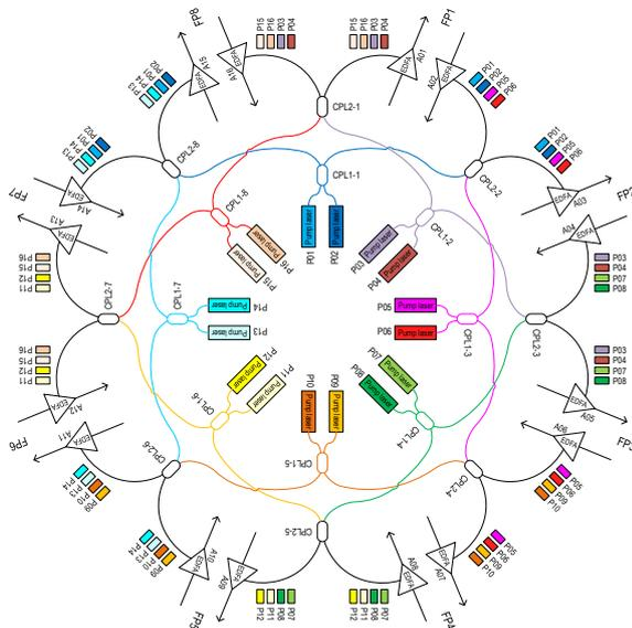
**Figure 8: 8FP Repeater Pump-redundancy Scheme**
