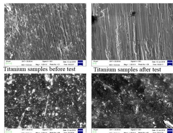
**Figure 2: Macroscopic morphology before and after test in simulated sea water for 72h**
