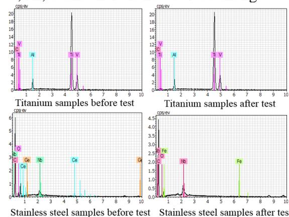
**Figure 3: EDS before and after test in simulated sea water for 720h**
