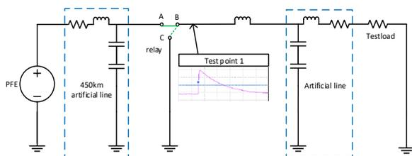
**Figure 5: Surge current test system**
