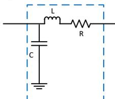
**Figure 2: Unit of the artificial line**
