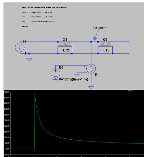
Figure 1: Surge simulation model and result in LTSPICE
