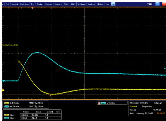
Figure 12: 15kV hot switch test result
