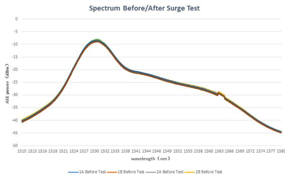
**Figure 9: Optical spectrum before and after surge test**
