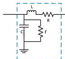
**Figure 3: Optimized unit of the artificial line**
