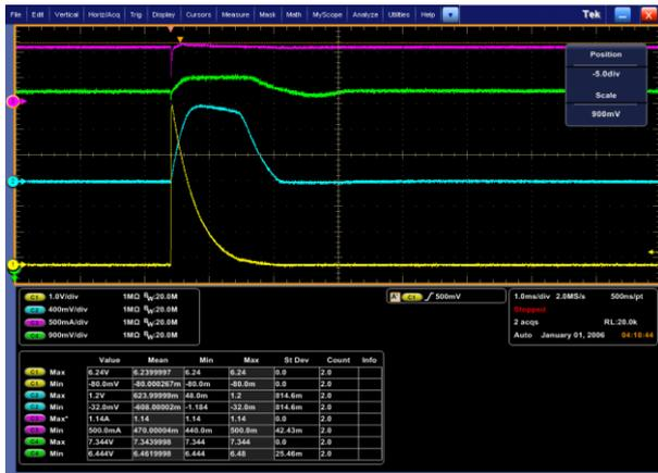
**Figure 8: Surge current protection test result**
