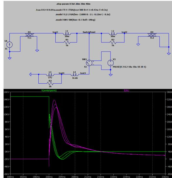
**Figure 10: Hot switch simulation model and result in LTSPICE**
