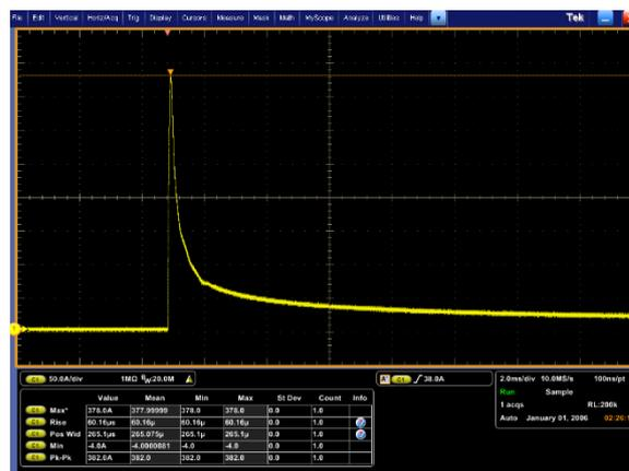
**Figure 5: Surge current test result on artificial line**
