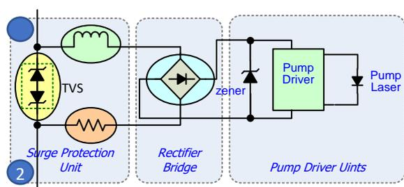
**Figure 6: Function unit of repeater**
