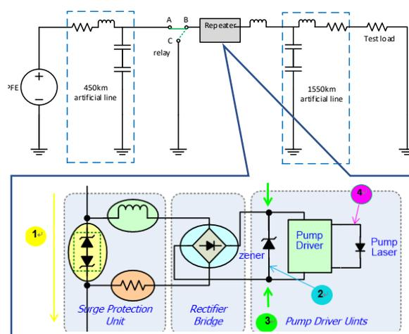
**Figure 7: Repeater surge protection unit test system**
