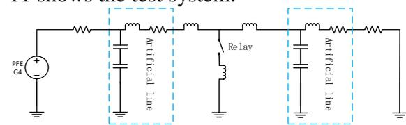
**Figure 11: 15 kV hot switch test on artificial line system**
