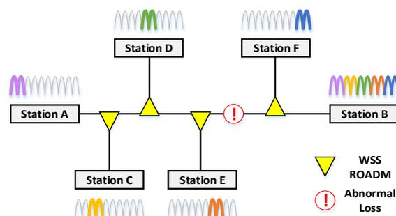
**Figure 3: An abnormal loss occurs in a submarine cable system with multiple WSS ROADM**
