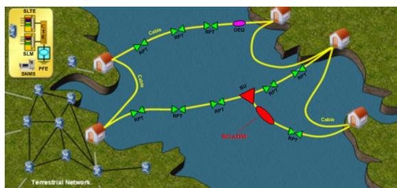
**Figure 1: Application of the ROADM in the submarine cable system**
