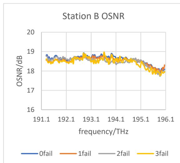
**Figure 9: The received OSNR of the B station after using the WSS ROADM's**
