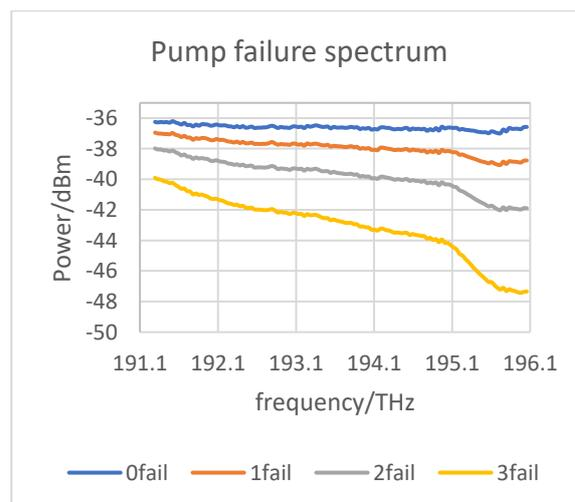
**Figure 5: The output power spectrum of repeater when pump failures occur**
