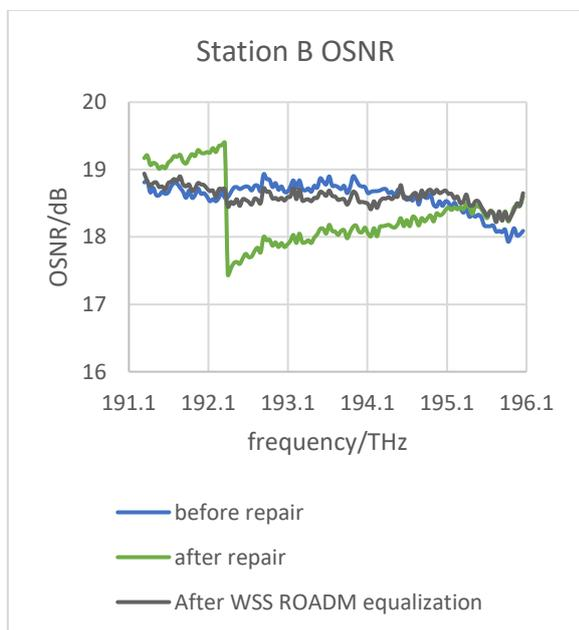
**Figure 11: The received OSNR of the B station before and after using the WSS ROADM's active gain shape equalization function after a submarine cable maintenance**
