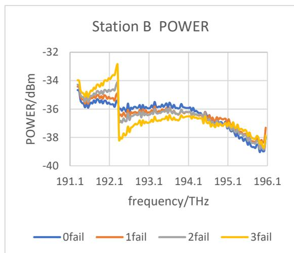
**Figure 6: The received power spectrum of the B station when pump failures occur in the repeater**
