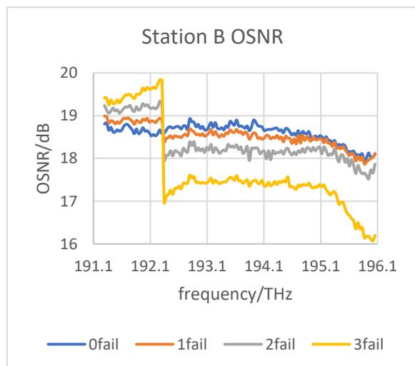
**Figure 7: The received OSNR of the B station when pump failures occur in the repeater**
