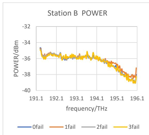
**Figure 8: The received power spectrum of the B station after using the WSS ROADM's active gain shape equalization function when pump failures occur in the repeater**
