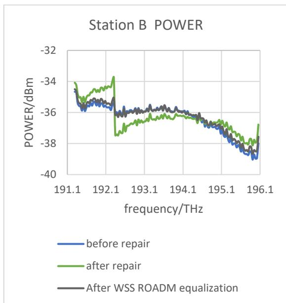
**Figure 10: The received power spectrum of the B station before and after using the WSS ROADM's active gain shape equalization function after a submarine cable maintenance**
