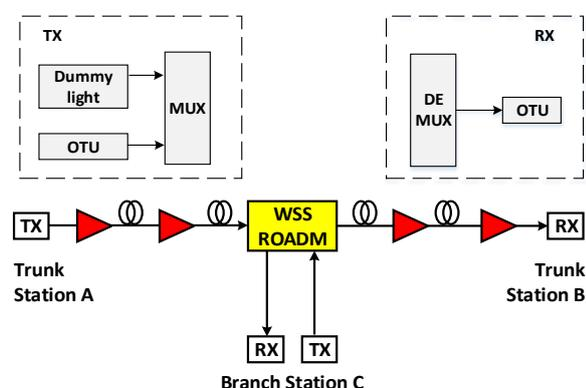
**Figure 4: The WSS ROADMs transmission system with a typical 3 stations**
