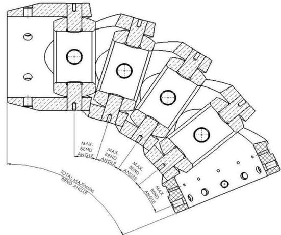
**Figure 12: Composite Bend Limiter Max Bend Angle**
