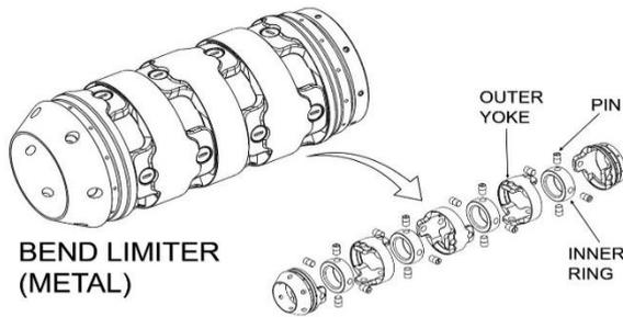
**Figure 10: Metal Bend Limiter**
