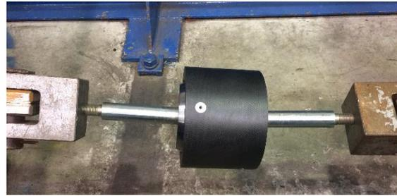
**Figure 8 Tensile test of Outer Yoke**
