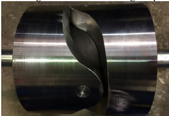
**Figure 7: Tensile test of Inner Yoke**
