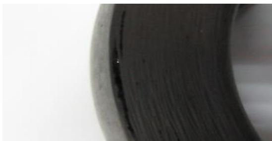
**Figure 4: Interlayer Defect**
