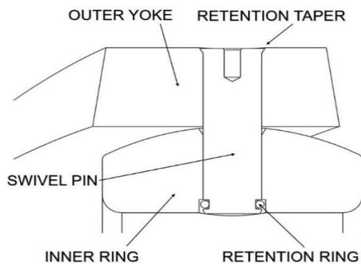
**Figure 15: Pin Retention**
