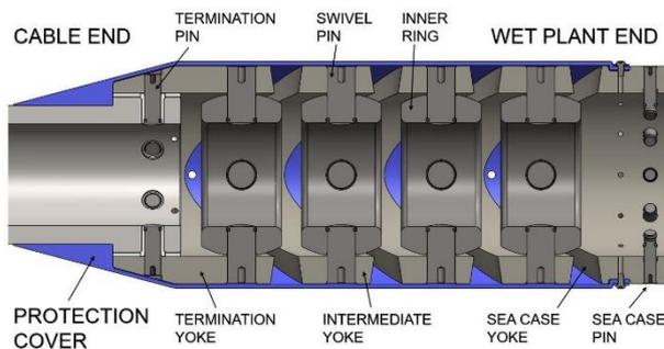
**Figure 11: Composite Bend Limiter Section**
