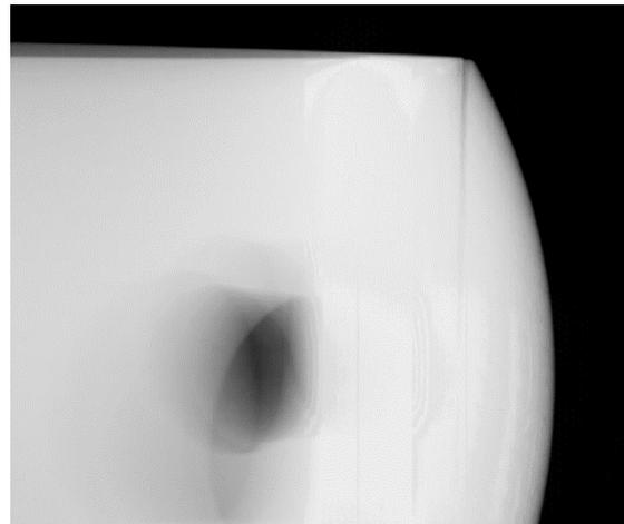
**Figure 5: X-ray image of Interlayer Defect**
