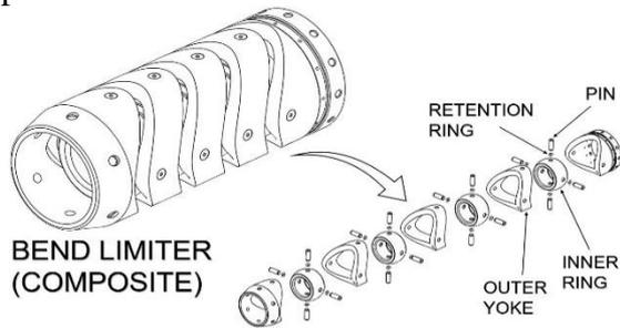
**Figure 9: Composite Bend Limiter**
