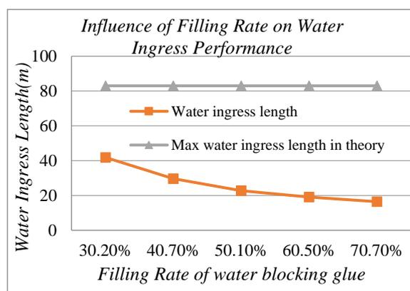
**Figure 8: Influence of filling rate of water blocking glue on water ingress performance**
