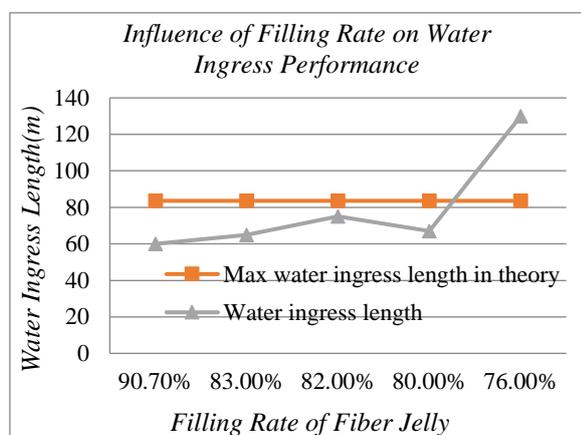
**Figure 7: Influence of filling rate of fibre jelly on water ingress performance**
