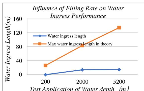
**Figure 9: Water ingress performance evaluation in different water depth**
