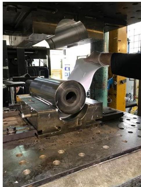
**Fig. 2 Wrapping of Sheet Material Around the Required Diameter Prior to Compression Moulding**
