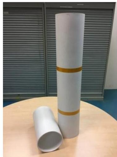
**Fig. 5 Silicone Liner in Three Sections for Initial Thermal Trial**
