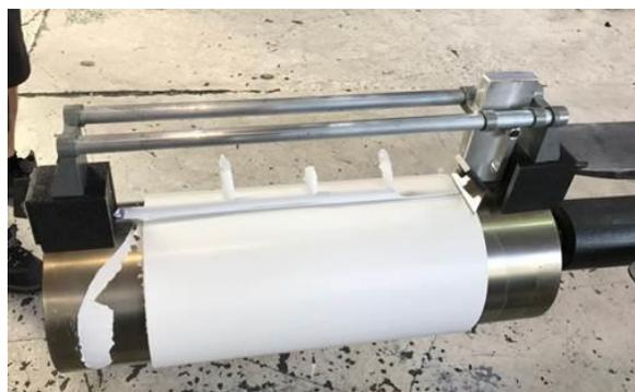
**Fig. 3 Machining Away of Surplus Material After Compression Moulding**
