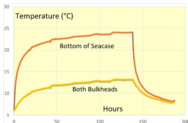
**Graph 2: Temperatures at Seacase Bottom and Bulkheads**
