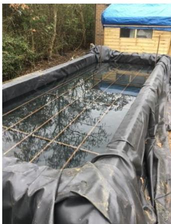
**Fig. 6: Constant-Temperature Water Bath, Prior to Covering**
