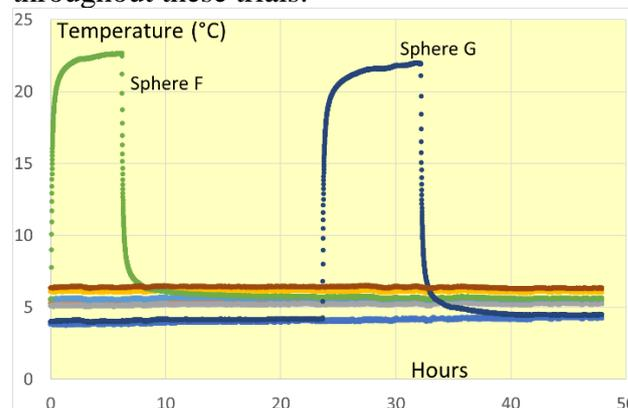
**Graph 1: Temperature Rises on Powering of 2 of the Sensor Spheres**
