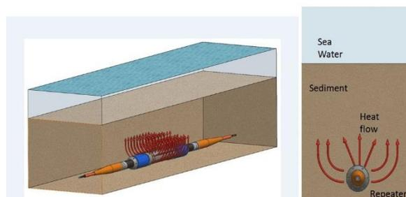
**Fig. 1: Thermal Flow from a Buried Repeater**
