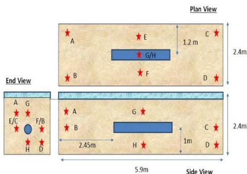
**Fig. 7: Positions of Thermal Conductivity Sensor Spheres**
