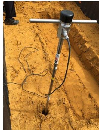
**Fig. 9: Calibrated Conductivity Probe in the Burial Sand**
