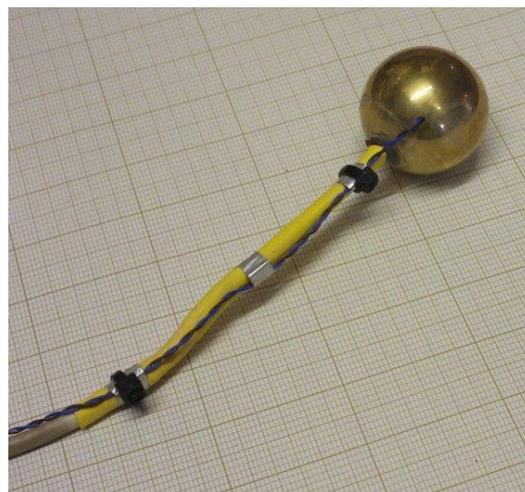
**Fig. 8: Thermal Conductivity Sensor Sphere**
