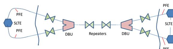
**Figure 1: The Duplicating Branching Unit showing two backhaul options**
