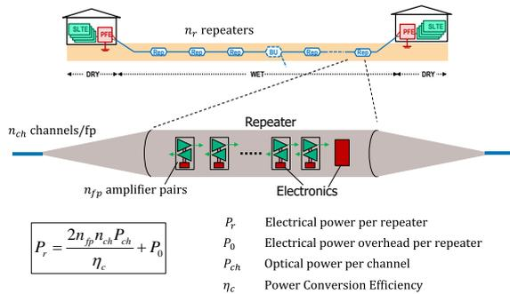
**Figure 3: Relation between the optical channel power and PFE power**
