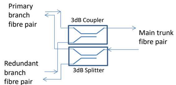
**Figure 2: Key optical elements within the DBU**
