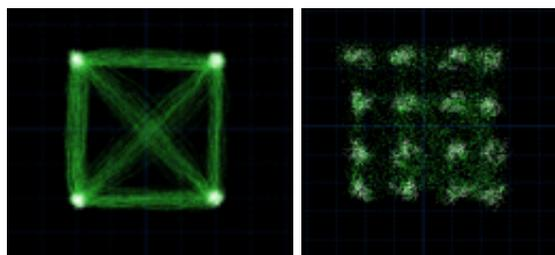
**Figure 1: Constellation diagrams of a QPSK signal on left and 16-QAM signal on right**
