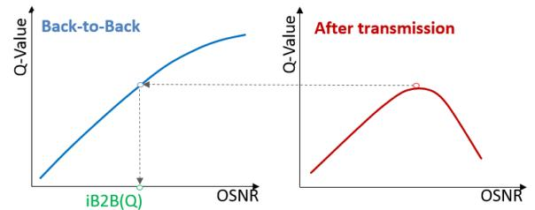
**Figure 2: Method of Obtaining  $iB2B(Q)$**
