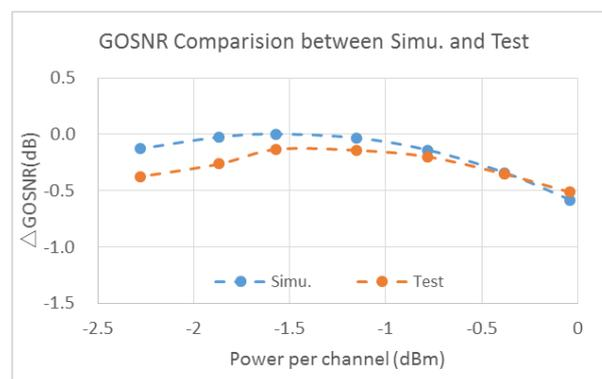
**Figure 6: Power vs  $\Delta$  GOSNR for Test and Simulation**
