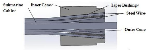
**Figure 3: Armoured steel wire clamping device**
