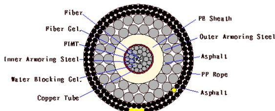
**Figure 1: Structure of the double armoured submarine cable**
