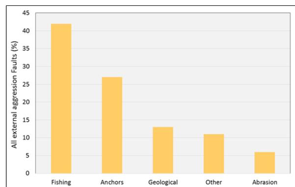
Figure 3: External aggression faults for all water depths (GMSL) [6].
