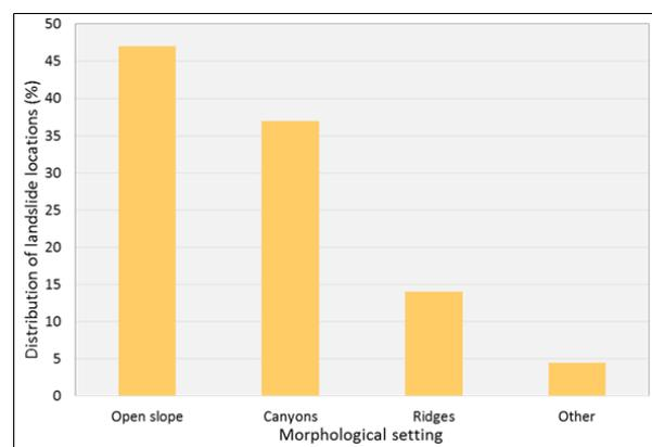
Figure 2: Distribution of landslide locations for the same sites [1][2]
