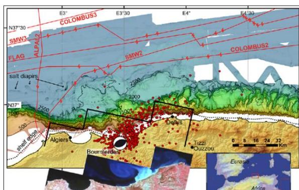
**Figure 4: Cable break distribution (red symbols) after the 2003 Boumerdès earthquake in the central Algerian margin. Red circles represent the location of the associated aftershocks. Only the most distal cable, COLOMBUS3, located in the abyssal plain, 80km away from Algerian coast, remains operational [7].**
