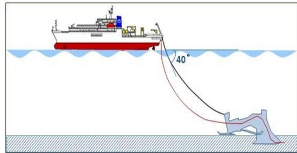
Figure 2: Plough tow wire angle
