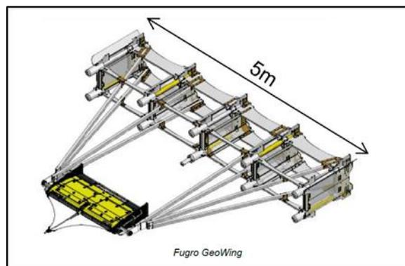
**Figure 1: Gradiometer from Fugro [4].**
