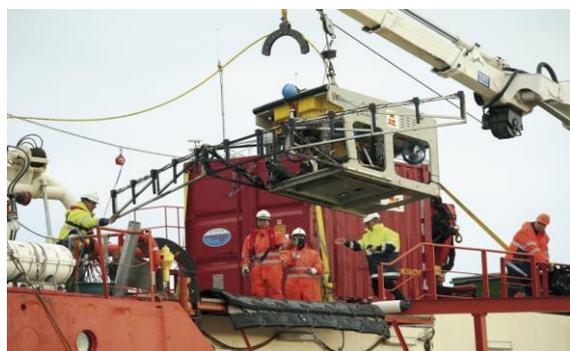
**Figure 2. Gradiometer framed ROV for Nord Stream Project [6]**
