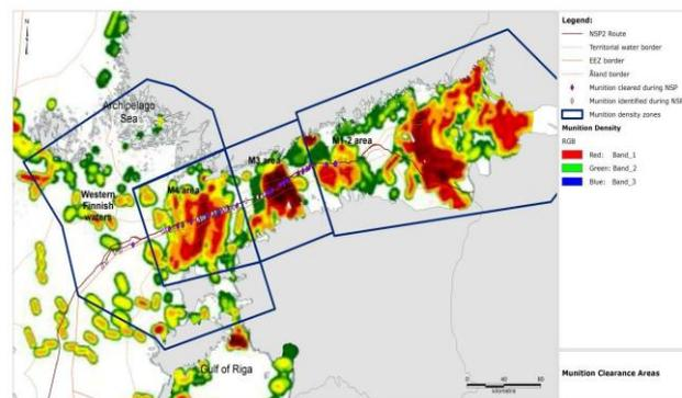
**Figure 3. UXO sensitivity assessment zones in Finnish part of the Nord Stream Project route [7]**
