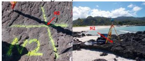
**Figure 3: One of Ground Control Point established on site**
