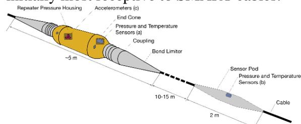
**Figure 9. The elements of a SMART cable**
