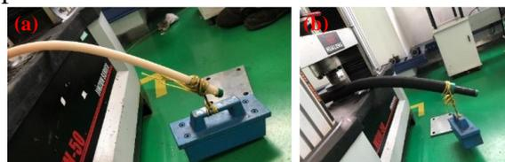
**Figure 10. Bending test on the high stiffness hose**
