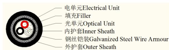
**Figure 2. The armored twin-conductor optical-electrical cable**
