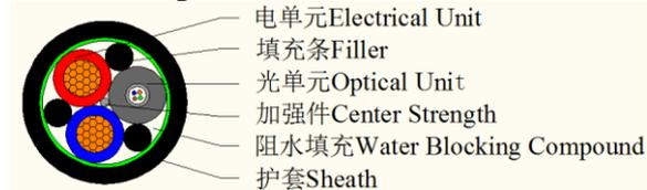
**Figure 3. The non-armored twin-conductor optical-electrical cable**
