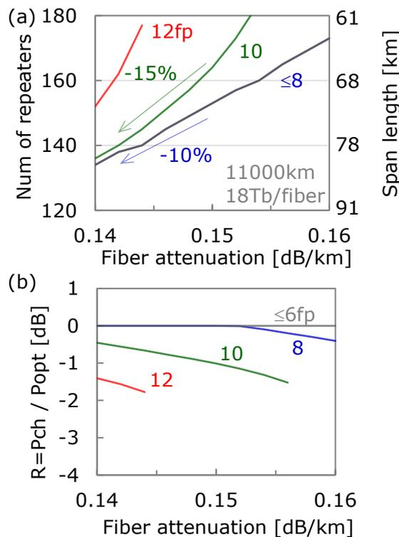
**Figure 4: Merit of low attenuation in reducing the number of repeaters (a), and nonlinearity ratio (b). The truncated solid lines mean upper limits of attenuation to achieve the target fiber capacity.**
