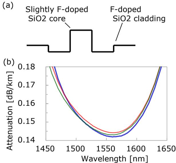
**Figure 1: Schematic structure of ultra-low loss Ge-free silica core fiber (a) and attenuation spectra of its samples with 12–50 km spools (b).**
