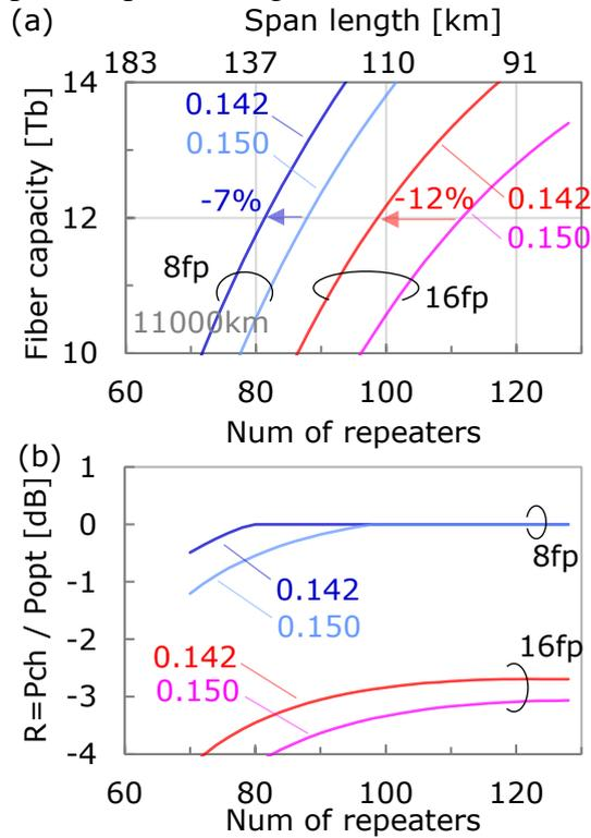
**Figure 2: Fiber capacity under power limitation as a function of the number of repeaters (or span length) (a), and difference in nonlinearity ratio (b) that illustrates difference between conventional nonlinear optimum regime (8fp) and power optimum regime with reduced signal power (16fp).**
