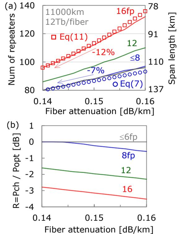
**Figure 3: Merit of low attenuation in reducing the number of repeaters (a), and nonlinearity ratio (b). Solid lines show results of numerical calculation, and plots show the approximate formulae for number of repeaters in nonlinear optimum (eq (7)) and power optimum (eq (11)) regimes.**
