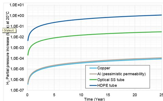
**Figure 8: Extract of paper study – Hydrogen partial pressure built up over time in optical tube, copper and aluminium conductors**
