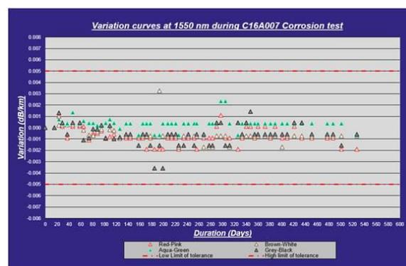
Figure 6: Optical follow-up at 1550nm during corrosion test
