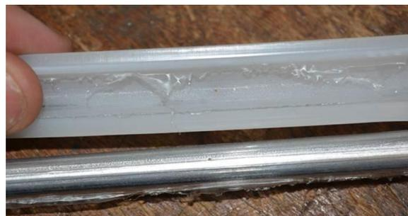
**Figure 12: Sample dissection after corrosion test on cable sample with shunt fault**
