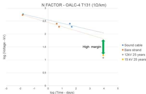
**Figure 7: N-factor statistical study of aluminium conductor cable, with and without bare strand (references [3] & [4])**
