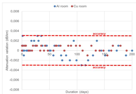
**Figure 10: Testing results for hydrogen transversal tightness test**
