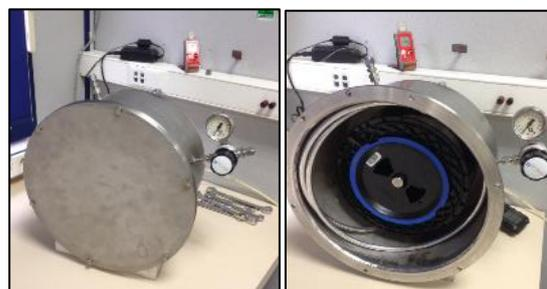
**Figure 9: Testing enclosure for hydrogen transversal tightness test**
