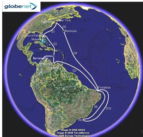
**Figure 1: Globenet's System Topology**
