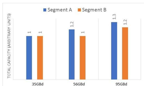
**Figure 3: Capacity per FP on two segments as function of modem technology**
