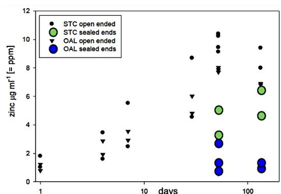
**Figure 5.** UK leachate results over 133 days for Zn released from DA cables by OAL and STC makers (Fig. 1). Most amounts peaked ~75 days after which
