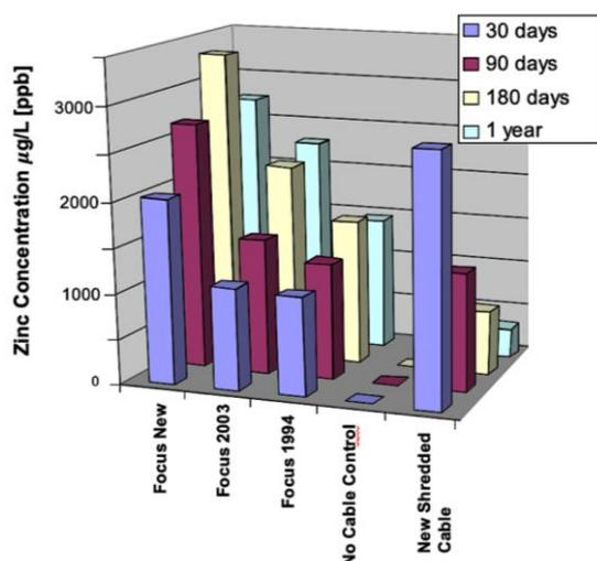
**Figure 6. Dissolved Zn from various types of LWA cable over time<sup>[8]</sup>; ppb = parts per billion. Graph NESDI.**
