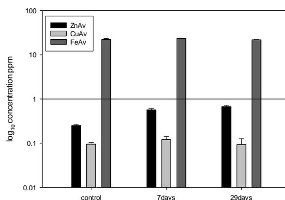
**Figure 4.** Zn, Cu and Fe in a seawater “control” tank without cables and tanks with LW cables that were analysed after 7 and 29 days<sup>[7]</sup>. A slight increase of 0.4ppm in Zn may reflect cross contamination from a DA cable during sample storage.
