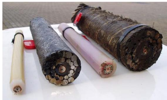
**Figure 1. Fibre-optic cable samples used for the UK leaching study<sup>[7]</sup> including (left to right) unarmoured Light Weight (LW) and Double Armoured (DA) cables from Alcatel (OAL-C4), and LW and DA samples from the now defunct Standard Telephone and Cables.**
