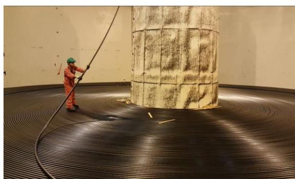
**Figure 3.** The general external condition of the HAW-3 cable is evident as it was stowed on the recovery vessel. Image ASN.
