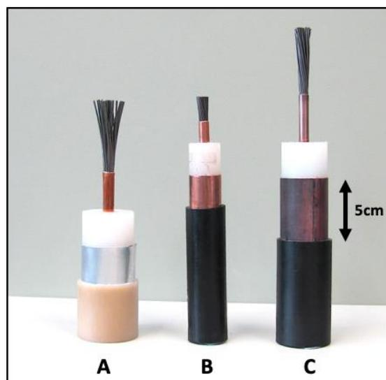
**Figure 7. Recovered coaxial cables highlighting condition of components after 38-44 years on the seabed. Samples are A. TAGIDE, B. FRANCE-MOROCCO-1 and C. HAW-3. Image L. Carter.**
