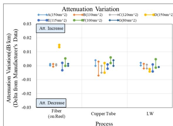
**Figure 4. Attenuation Variation During Cabling (12 fiber pairs)**
