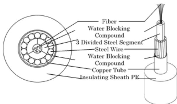
**Figure 1. OCC-LW (Light Weight) cable structure**
