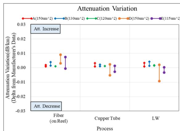
**Figure 3. Attenuation Variation During Cabling (16 fiber pairs)**
