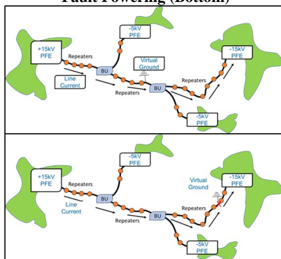
PFE typically operates in current regulation mode. The PFE current is set to the line current required to power the system and the voltage automatically balances to the virtual ground of the system. When a voltage limit is reached, for example when SEF is not supported and a shunt fault occurs, the PFE switches to voltage regulation mode. In voltage regulation mode, the PFE will maintain a constant voltage and the line current will decrease until the proper system powering condition is met.
