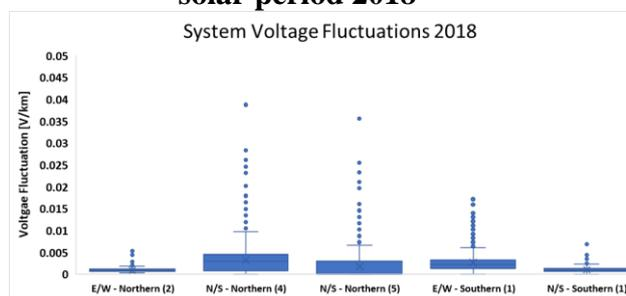
Clearly, the voltage fluctuations experienced during the non-active solar flare period are less than those experienced during the 2017 solar events. Voltage fluctuations on three newer systems, installed and commissioned after 2015, were also studied during the non-active solar period in 2018. The data for these new systems is shown in Figure 7.
