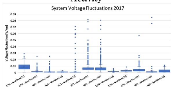
Further observations of the data for the legacy systems shows that the largest voltage fluctuation of 0.085 V/km occurred on N/S –
