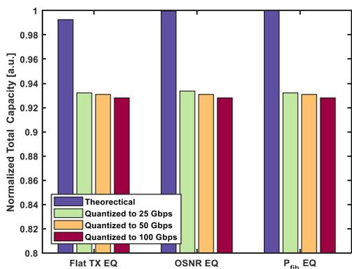
**Figure 12: The total system capacity based on the measured eSNR for various**
