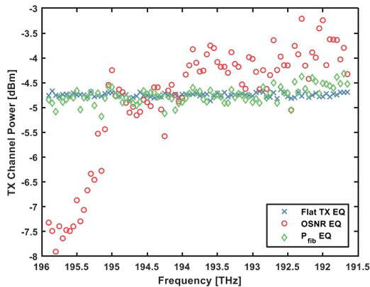
**Figure 3: The TX channel power spectrum of the different equalization methods for 6,300 km of propagation.**
