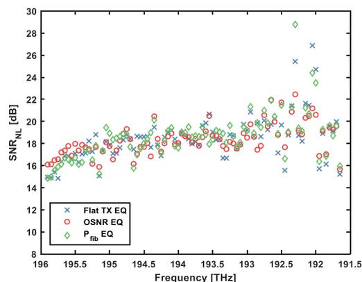
**Figure 5: The calculated SNR<sub>NL</sub> across the C-band for various equalization strategies after 6,300 km of propagation.**
