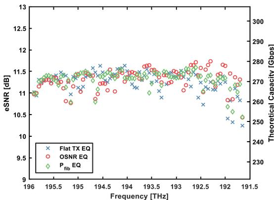
**Figure 4: The measured eSNR, as reported by the modem, across the C-band for various equalization strategies after 6,300 km of propagation.**
