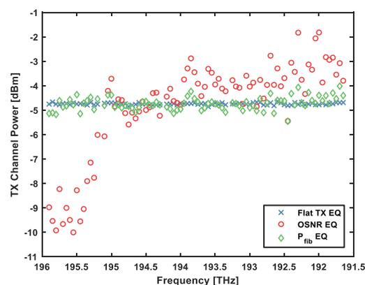
**Figure 9: The TX channel power spectrum of the different equalization methods for 12,600 km of propagation.**
