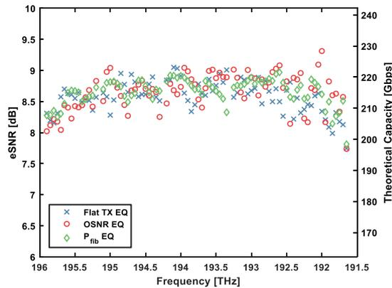
**Figure 10: The measured eSNR, as reported by the modem, across the C-band for various equalization strategies after 12,600 km of propagation.**
