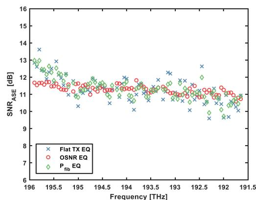
**Figure 8: The measured SNR<sub>ASE</sub> across the C-band after 12,600 km of propagation for various equalization methods.**
