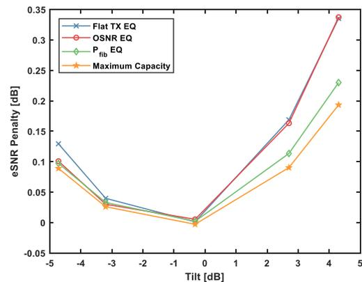
**Figure 1: The simulated effect of gain tilt on eSNR penalty averaged across the C-band for different equalization strategies. Max capacity equalization is based on a "brute force" method determined through iterative optimization techniques.**
