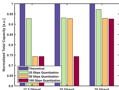
**Figure 7: Total system capacity interpolated for different baud rates under flat TX equalized conditions after 6,300 km of propagation. Normalizations are relative to the theoretical capacities.**
