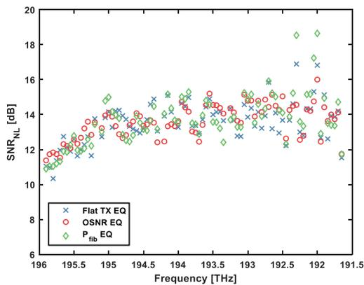
**Figure 11: The calculated SNR<sub>NL</sub> across the C-band for various equalization strategies after 12,600 km of propagation.**
