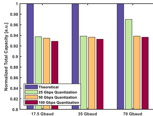
**Figure 13: Total system capacity interpolated for different baud rates under flat TX equalized conditions after 12,600 km of propagation. Normalizations are relative to the theoretical capacities.**
