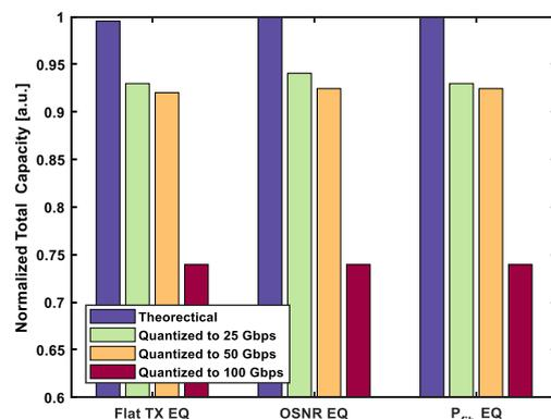
**Figure 6: Normalized total system capacity based on the measured eSNR for various equalization strategies, and quantization step sizes after 6,300 km of propagation.**
