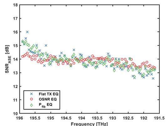
**Figure 2: The measured  $SNR_{ASE}$  across the C-band after 6,300 km of propagation for various equalization methods.**
