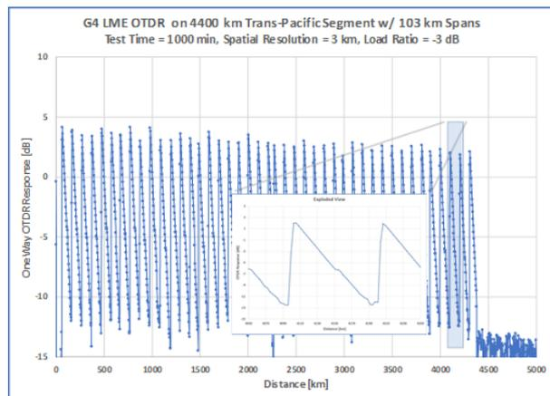
**Figure 2: 103km LME-OTDR span visibility**
