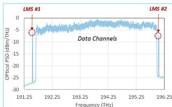
**Fig 1b: LMS Probe Tones in the Tx Band**
