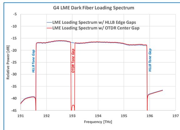
**Figure 4: Embedded ASE Loading spectra for dark-fiber measurements**
