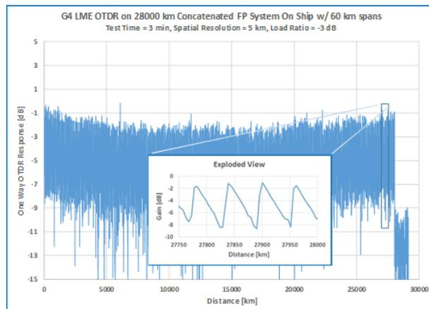
**Figure 3: LME-OTDR on a 28000 km system**
