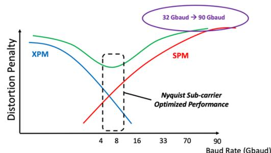
**Figure 2: Optimum baud rates for transmission.**
