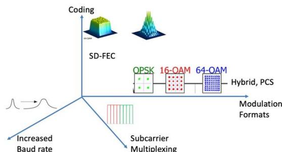
**Figure 1: Four optimization axes of SLTE techniques for increasing capacity.**
