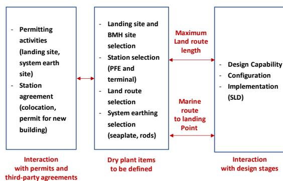
**Figure 6: Interactions between dry plant definition, overall design stages, and permitting activities**
