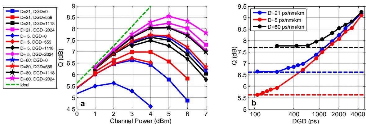
**Figure 2: Large PMD fiber simulation results. a) Q versus channel power for different levels of DGD, for fibers with three different dispersion parameters, 21 ps/nm/km (square), 5 ps/nm/km (diamond), and 80 ps/nm/km (stars). DGD has units of ps. Green line shows the ideal Q value expected due to the received SNR from amplifier noise only. b) Maximum Q versus DGD for the three chromatic dispersion values. Dashed lines show the maximum Q for DGD=0.**
