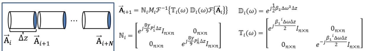
Figure 1: Schematic explaining the modeling of the nonlinear transmission in the LPMD fiber and CC-MCF fiber.
