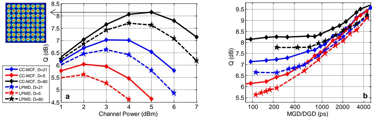
**Figure 3: Comparison of CC-MCF to large PMD fiber. a) Q versus channel power with both MGD=DGD=0, and for three different dispersion parameters, 21 ps/nm/km (blue), 5 ps/nm/km (red), and 80 ps/nm/km (black). b) Maximum Q versus MGD for three different dispersion values.**
