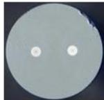
125 $\mu\text{m}$ cladding |
