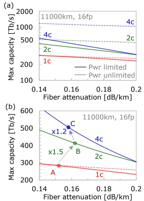
**Figure 1: Theoretical maximum capacity as a function of fiber attenuation and the number of cores (a), and its magnified view (b). Plots A, B, and C shows the current fiber, U-2CF, and C-4CF, respectively.**
