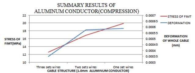
Figure 13: Summary Compression Results of Aluminium Conductor (1.0mm)
