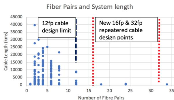
Figure 5: Cable System Length Versus Number of Fibre Pairs
