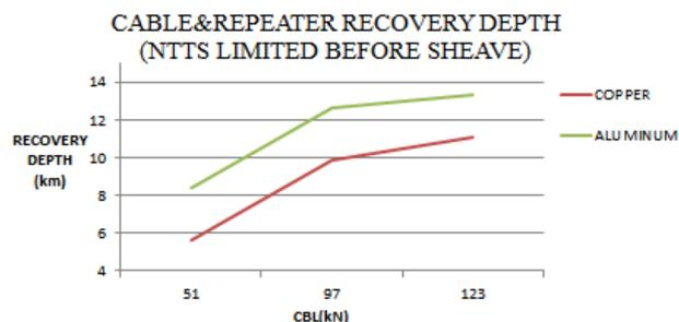
Figure 24: Cable & Repeater Recovery Depth (NTTS Limited Before Sheave)
