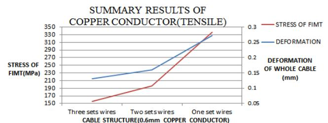
Figure 15: Summary Tensile Results of Copper Conductor (0.6mm)
