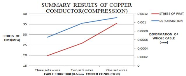
Figure 14: Summary Compression Results of Copper Conductor (0.6mm)
