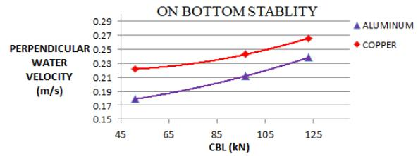
Figure 19: LW Cable Bottom Stability
