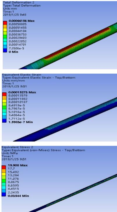
Figure 17: Simulation Results for Three Sets Wires Using 0.6mm Copper Conductor (Compression)
