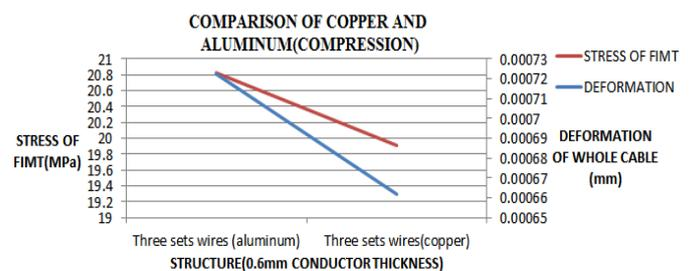
Figure 16: Comparison of Compression Results Between Copper and Aluminium
