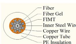
Figure 11: Copper Wire & Tube
