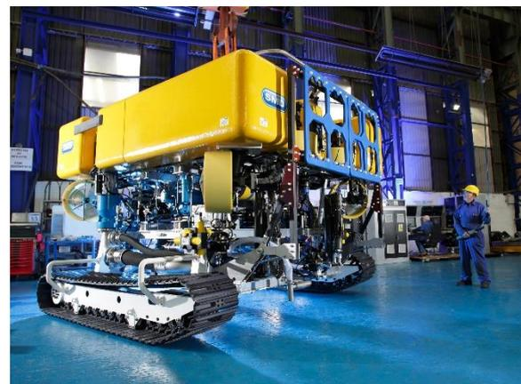
**Figure 3: 500HP Trenching ROV - QT500**
