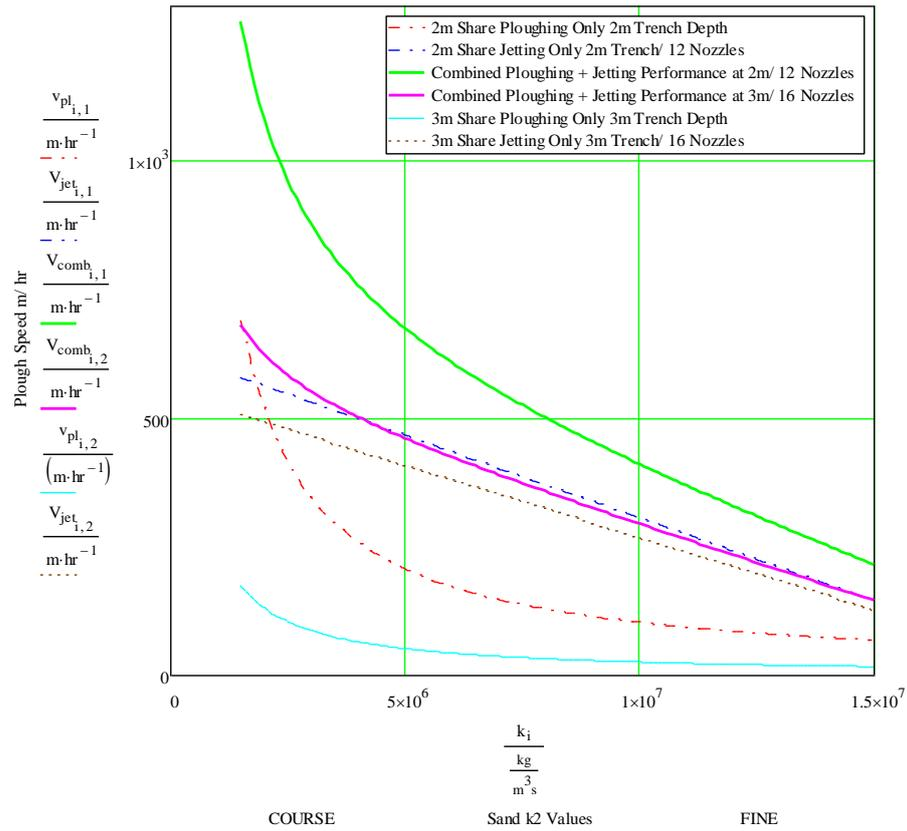
**Figure 6 - MD3 Plough Speed (m/hr) for 3 Sand Relative Density Conditions**
