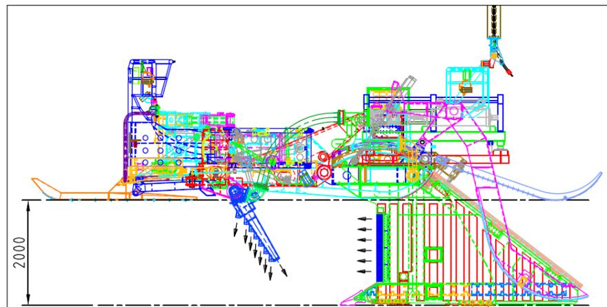
Figure 4 - MD3 shown in 3.0m burial mode; front jet tool deployed and jetting through share leading edge and under heel
