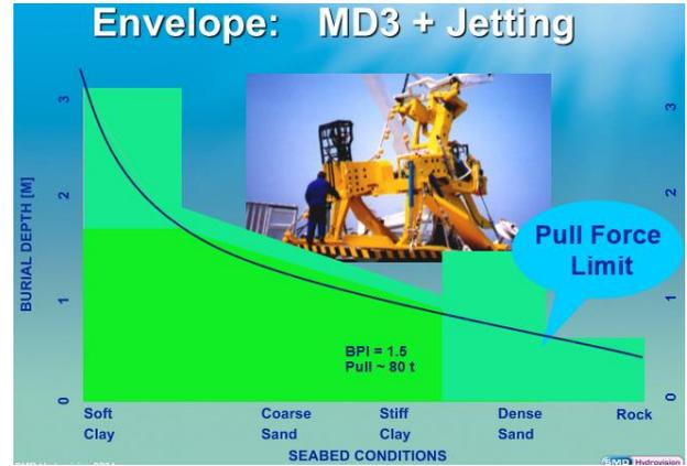
Figure 2 - Performance Envelope of MD3 with Jetting Assist
