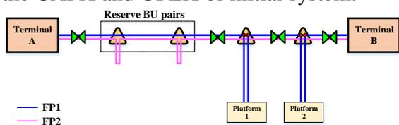
**Figure 9: Initial Network Architecture for BU Pairs Solution**
