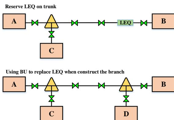
**Figure 4: LEQ Solution Before and After Branch Installation**
