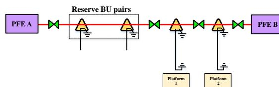
**Figure 10: Initial Power Feeding Configuration for BU Pairs Solution**
