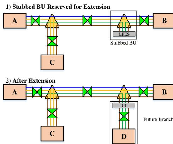
**Figure 2: Stubbed BU Solution Before and After Extension to Station D**
