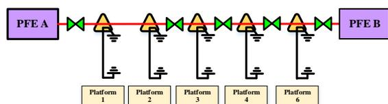
**Figure 6: Power Feeding for OADM BU Solution for Oil & Gas Platform Application**
