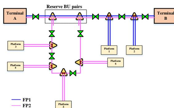
**Figure 11: Network Architecture after Extension for BU Pairs Solution**
