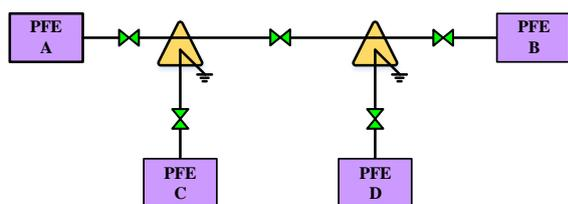
**Figure 3: Power Feeding Configuration After the Extension to Station D**
