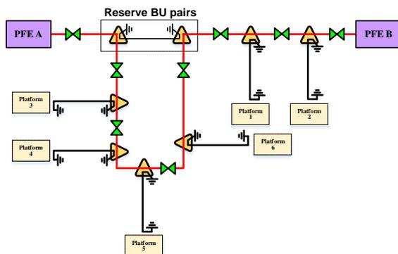
**Figure 12: Power Feeding Configuration after Extension for BU Pairs Solution**
