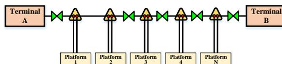
**Figure 5: OADM BU Solution for Oil & Gas Platform Application**
