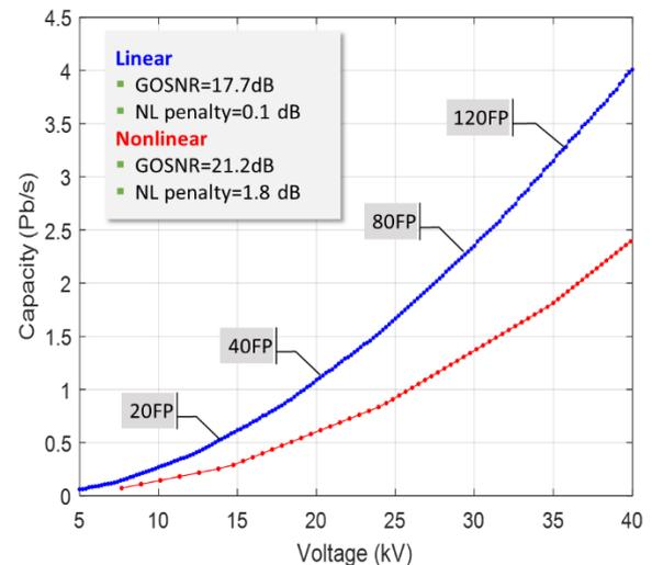
**Figure 4: Ultimate Capacity as a function of Voltage for linear (blue) and nonlinear (red) systems.**
