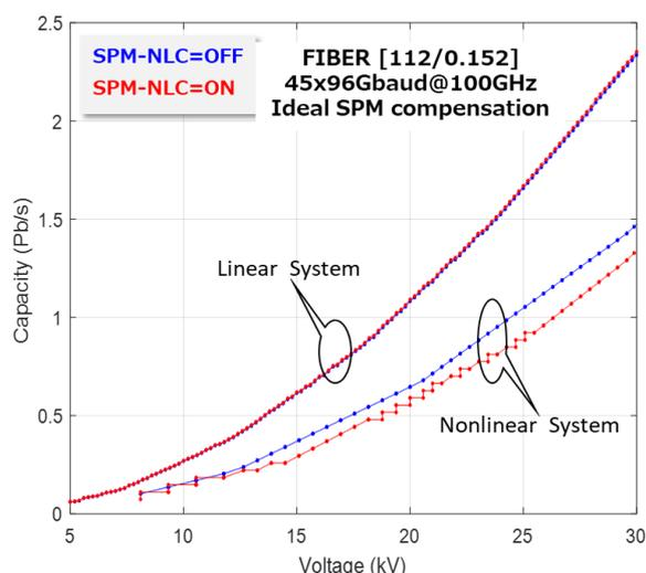
**Figure 7: Ultimate capacity for linear and nonlinear systems with and without ideal SPM compensation**
