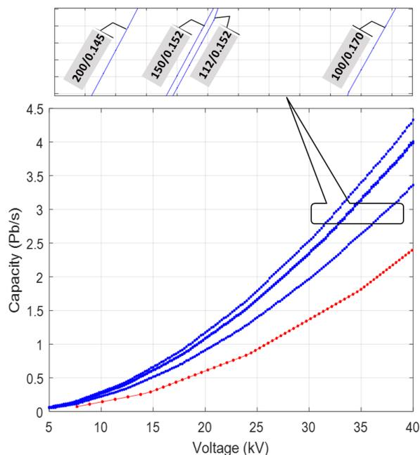
**Figure 5: Fiber dependency on ultimate capacity vs voltage**
