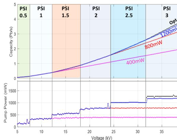
**Figure 6: Pump scheme dependency on ultimate capacity vs voltage**
