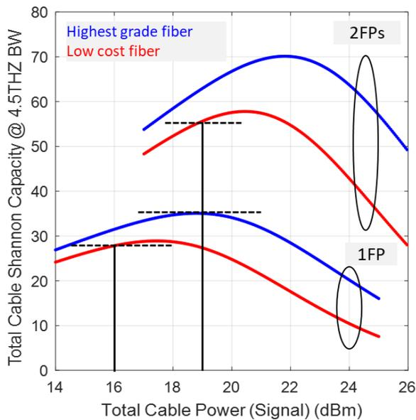
**Figure 2: Cable Capacity vs Total Cable Signal Power**
