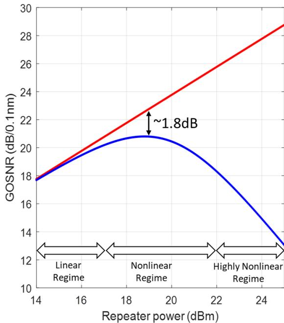
**Figure 1: OSNR and GOSNR (45 carriers) vs Repeater Power in a 10000km system**
