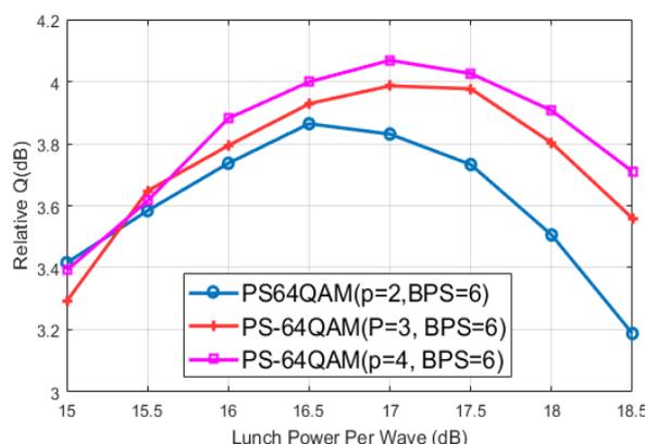
**Figure 1: Measured super-Gaussian nonlinear performance for 4000 km of uncompensated Tera Wave fiber at PS-64QAM BPS=6 bits.**
