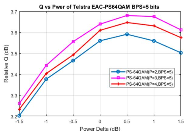
**Figure 4: Measured super-Gaussian nonlinear performance for 3000 km of compensated Telstra fiber at PS-64QAM BPS=5 bits.**
