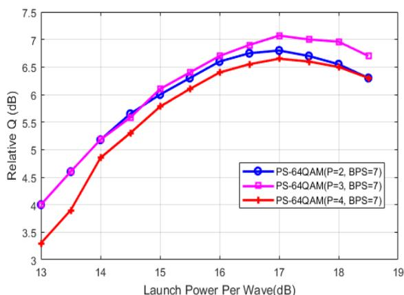
**Figure 2: Measured super-Gaussian nonlinear performance for 4000 km of uncompensated Tera Wave fiber at PS-64QAM BPS = 7 bits.**
