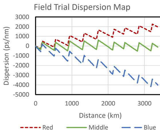
**Figure 3: Field trial dispersion map contains a zero-dispersion window near the middle of the spectrum. The legacy cable impacts higher nonlinearity penalties to coherent carriers compared to newer cables with TeraWave fiber.**
