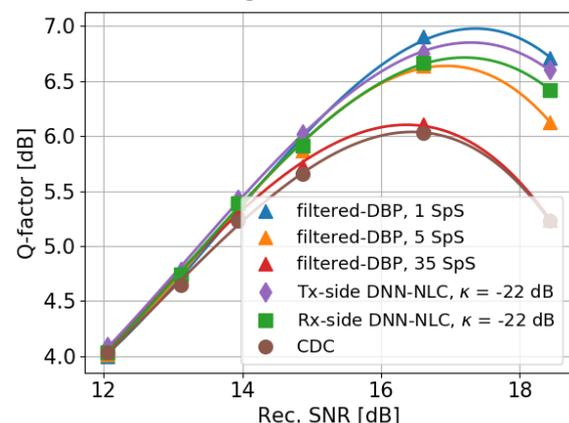
**Fig. 7 The performance comparison between NN-NLC at transmitter and receiver side, and filtered-DBP at different spans per step for single-channel DP-16QAM after 2800 km**
