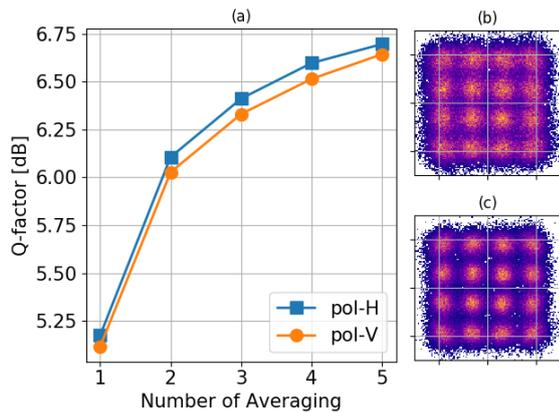
**Fig. 3 The impact of de-noise averaging of the training datasets on the Q-factor at SNR = 18.4 dB after 2800 km**
