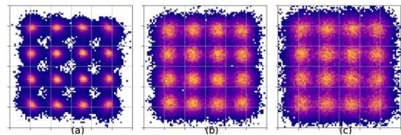
**Fig. 6 Pre-distorted symbols at transmitter side (a); recovered constellation at the receiver with (b) and without (c) transmitter-side NN-NLC. Received SNR = 18.4 dB@2800 km transmission.**
