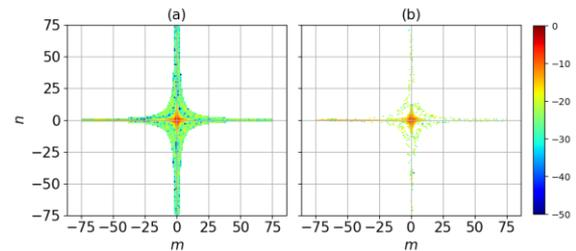
**Fig. 4 The density plot of the input layer weights of the NN model at initial  $N_t = 1929$  (a) and  $N_t = 615$  triplets after iterative trimming ( $\kappa = -22$ dB) (b).**
