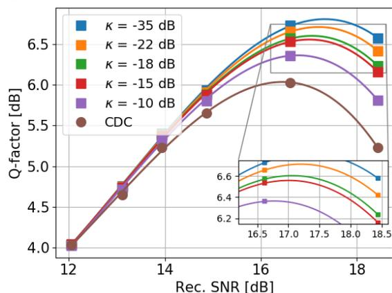
**Fig. 5 The impact of trimming threshold  $\kappa$  on the NN-NLC at the receiver side after 2800km transmission.**
