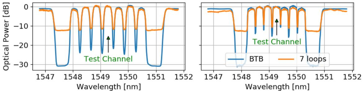
**Fig.2 (b) WDM Spectra at 50GHz (left) and 37.5GHz (right)**
