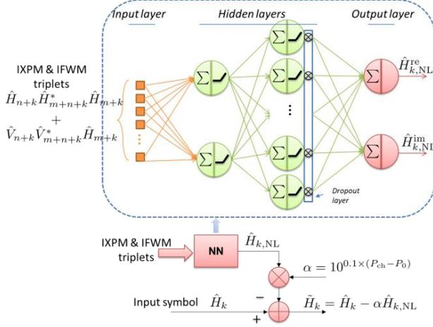
**Fig. 1 The block diagram of the proposed NN-NLC illustrated for pol-H only. The diagram in the dashed box describes the optimized NN architecture with 2 hidden layers used in the paper.**
