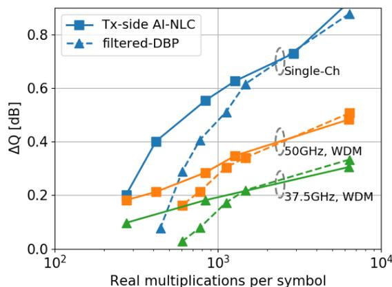
**Fig. 8 The comparison of Q-factor improvement between Tx-side NN-NLC and filtered-DBP. FFT size is assumed to be 4086.**
