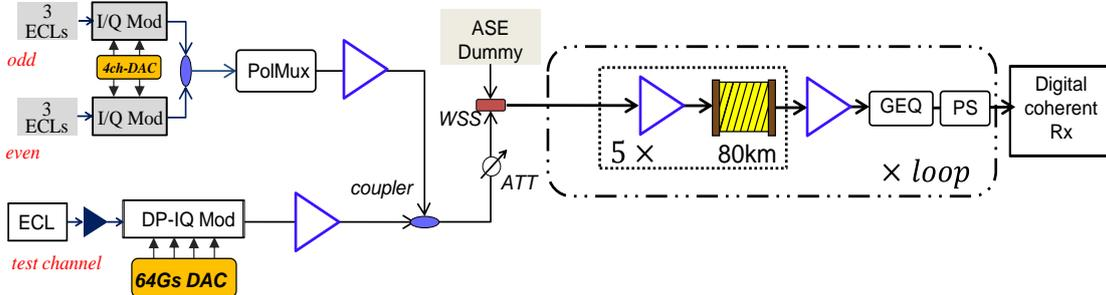
**Fig.2 (a) System setup of the transmitter and transmission loop. DAC: digital-to-analog converter, ECL: external cavity laser, GEQ: gain equalizer, PolMux: polarization multiplexer, PS: polarization scrambler, WSS: wavelength-selective switch.**
