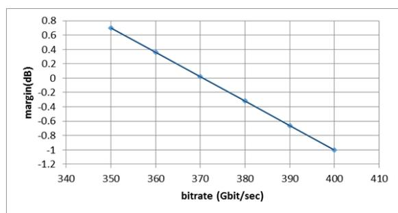
**Fig. 1.2. Non-allocated margin for design at 8000 km transmission distance**
