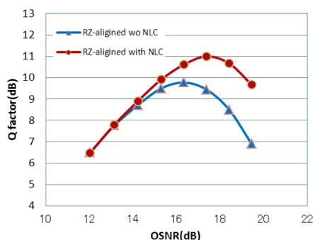
**Fig. 2.1. Transmission characteristics using nonlinear compensation**
