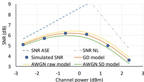
**Figure 2: numerically simulated combination of SNR<sub>ASE</sub> and SNR<sub>NL</sub>, for 34Gbd QPSK link [8].**
