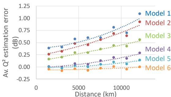
**Figure 3: Average Q<sup>2</sup> factor estimation error (whatever format, spacing, power) vs distance on 36nm loop test-bed, with XWAV transceivers**
