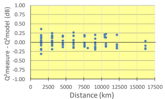
**Figure 4: Q<sup>2</sup> factor error versus distance, for all configurations described in section 4.**
