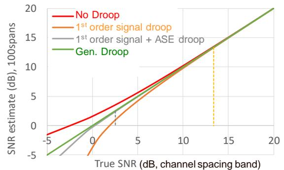
**Figure 1: SNR<sub>ASE</sub> estimations vs exact SNR computation, after a cascade of 100 repeaters. Exact SNR corresponds to Generalized Droop model, [4] and [3] (Eq. A4); “No Droop” corresponds to theoretical OSNR in Eq. 4; “1<sup>st</sup> order signal droop” corresponds to [3] (Eq. 4), and “1<sup>st</sup> order signal +ASE droop” to Eq. 6.**
