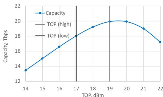
**Figure 2. Total Capacity versus TOP for 100km repeater spacing**
