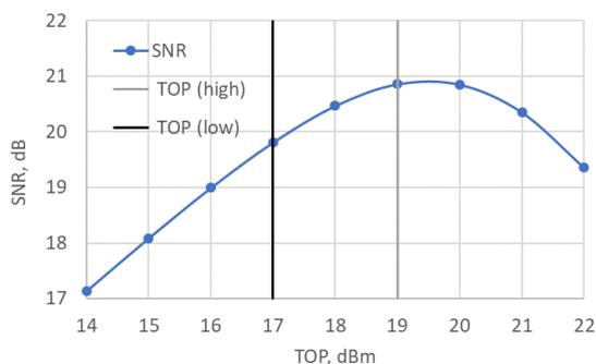
**Figure 1. SNR versus repeater TOP for 100km repeater spacing**
