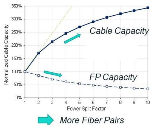
**Figure 5. Illustration of increasing cable capacity as more fiber pairs are added, using the SDM design approach.**
