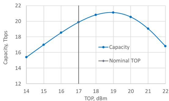
**Figure 3. Total Fiber Capacity versus TOP for 90km repeater spacing**
