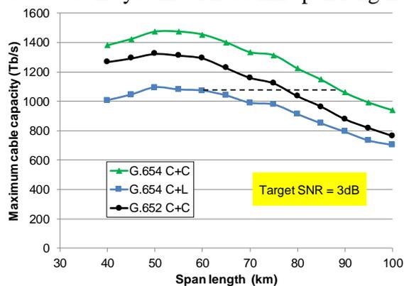
**Fig. 6: Cable capacity as a function of span length for a target SNR value of 3 dB and a 6,600 km link.**
