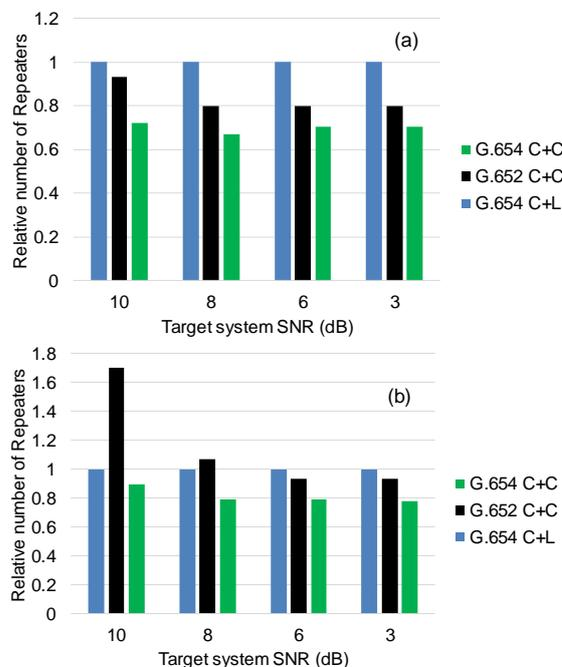
**Fig. 7: Relative number of repeaters needed for equal capacity systems with same target SNR values for link lengths of a) 6,600 km and b) 10,000 km.**
